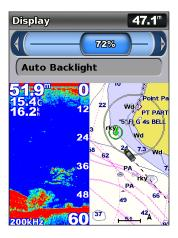
To allow the unit to automatically adjust the backlight based on ambient light, select **Auto Backlight** (automatic backlight is available only on the GPSMAP 526 and 556).
